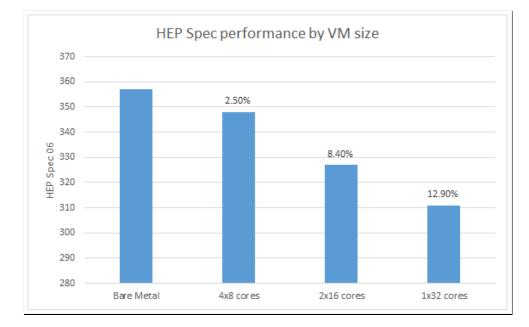
Results for other applications may vary so each option should be verified for the target environment. The percentages from our optimisations are not necessarily additive but give an indication of the performance improvements to be expected. After tuning, we saw around 5% overhead from the following improvements.
