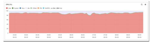
When EPT was turned off. some selected hypervisors showed a very difference performance profile. A major increase in non-user load and a reduction in the throughput for the experiment workloads. However, this effect was not observed on the servers with AMD processors.
