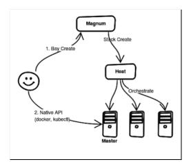
Magnum relies heavily on Heat for the orchestration part of the container clusters - called **bays**. Bays are instantiated based on pre-defined **bay models**, which set how the master and the other nodes should look like (flavor, image, etc) and which container orchestration engine (COE) should be used - among other possible configuration options. Current choices include Docker Swarm, Kubernetes and Mesos. The Magnum homepage gives a lot more details.
